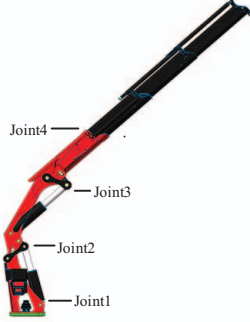
Figure 1. Structure of lifting arm
